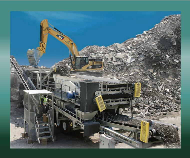
**6500LP PORTABLE IMPACT CRUSHING PLANT**
